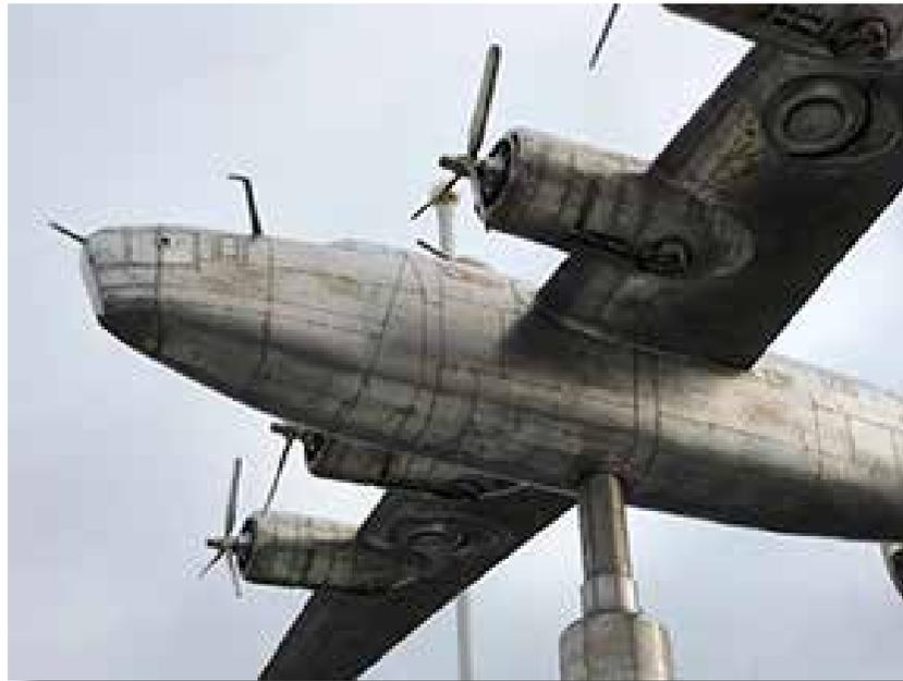
The cause of the rust appears to have been from Iceland's harsh weather, salt in the air and chemicals being released into the atmosphere through evaporation from the nearby Blue Lagoon Spa.
